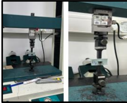
Figure 3: Determination of Tear Strength using Tensile Testing Machine
