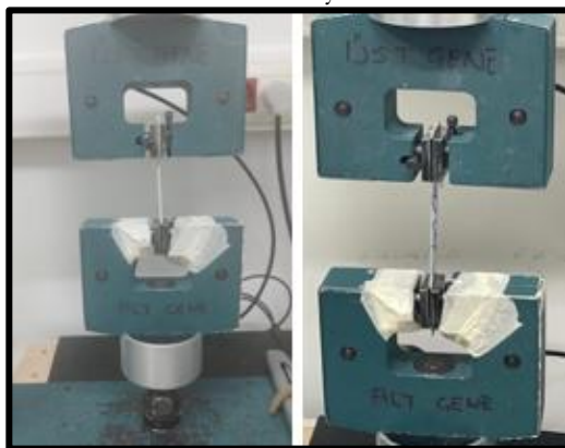
Figure 2: Determination of Tensile Strength and Elongation using Tensile Tester
