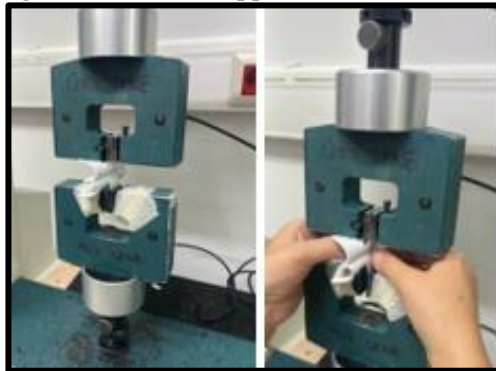
Figure 4: Determination of Seam strength using Tensile Testing Machine
