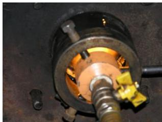
Fig. 9. Testing a hydrovortex atomiser at a mini oil refinery.
