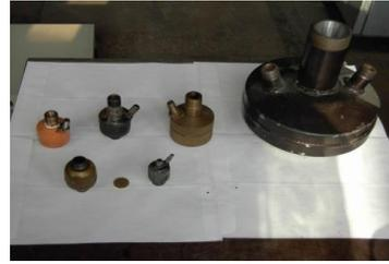
Fig. 5. Static pressure function ( $Re=1,000$ ,  $Eu = 10$ ). Fig. 6. Types of mixer atomisers
